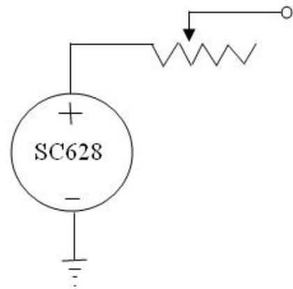
It was verified that the circuitry of model SC628R is not affected by a potentiometer, so data was gathered to find the value of a potentiometer that gives the greatest range of sound change.
