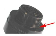
As the picture to the left shows, the locking flats are only located at the base of the nose ring. The locking flats do not extend up the side of the nose threads.
